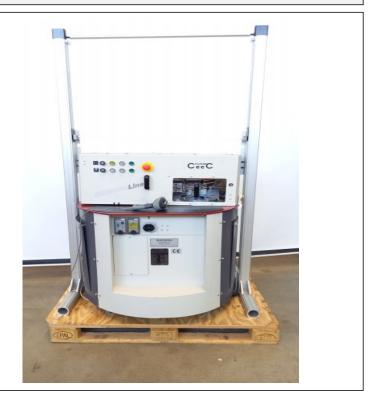
The FourC machine is for automatic measuring of gemstones which are not undercut during the rotation.
